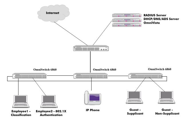
Figure 35-12 : Access Guardian Network Configuration Example
