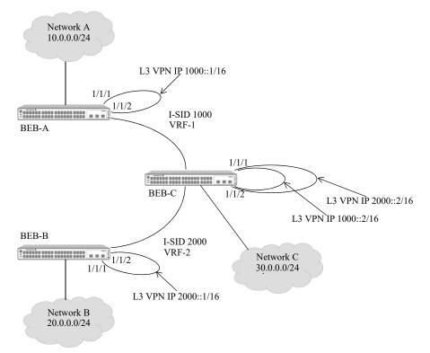
Figure 7-24 : IPv6 Inter-ISID Routing Example (Two VRFs)
