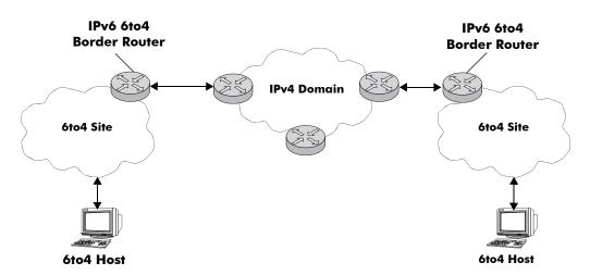
Figure 23-1 : Basic traffic flow between IPv6 hosts over IPv4 domain
