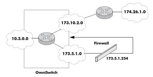
Figure 33-7 : Using a Built-In Port Group
