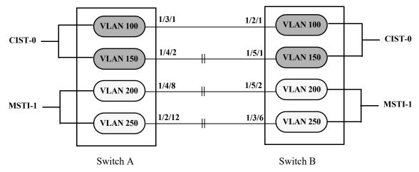
Figure 6-13 : Flat Mode MSTP Quick Steps Example
