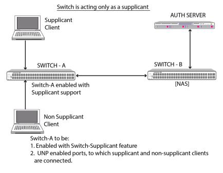
Figure 35-11 : Switch is acting only as a supplicant
