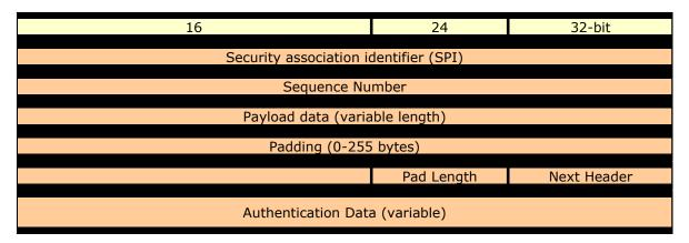
Figure 24-2 : IP Packet protected by ESP
