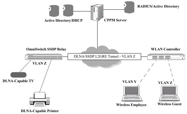
Figure 35-17 : SSDP - Wireless DLNA-Capable Clients
