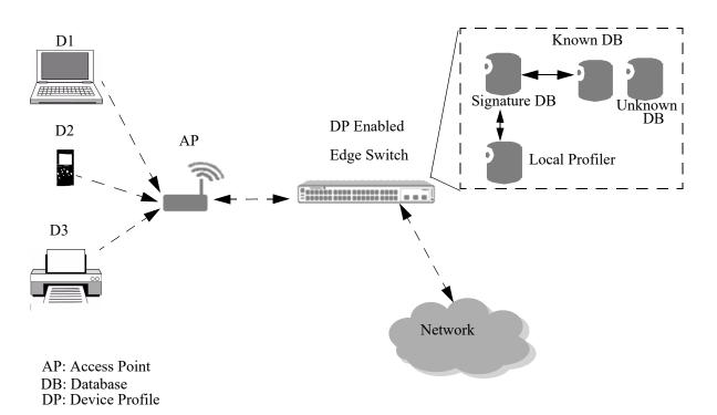
Figure 35-25 : IoT Device Profiling Overview
