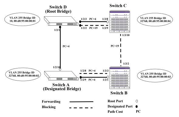
Figure 6-11 : Example Active Spanning Tree Topology
