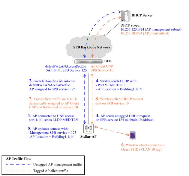
Figure 35-8 : OmniSwitch AP Discovery and Integration Example - SPB Domain
