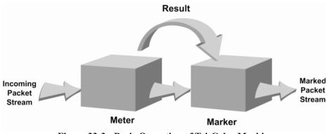
Figure 33-3 : Basic Operation of Tri-Color Marking
