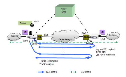
Figure 46-3 : CPE Test group Example - Unidirectional, Ingress Test
