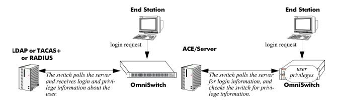
Figure 38-1 : Servers Used for Authenticated Switch Access
