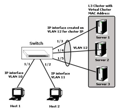
Figure 5-3 : Switch connected to an L3 Server Cluster through 3 ports (1/1/3,1/1/4,1/1/5)
