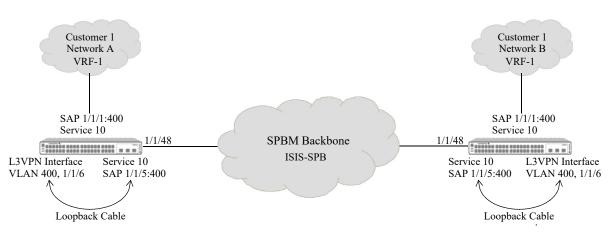
Figure 7-25 : L3 VPN Interface Before Migration to Inline Routing
