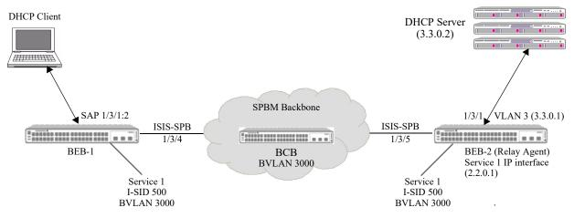
Figure 27-3 : Sample SPB Network Topology with DHCP Relay
