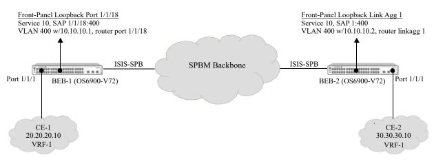
Figure 7-19 : L3 VPN Front-Panel Ports (Inline Routing)
