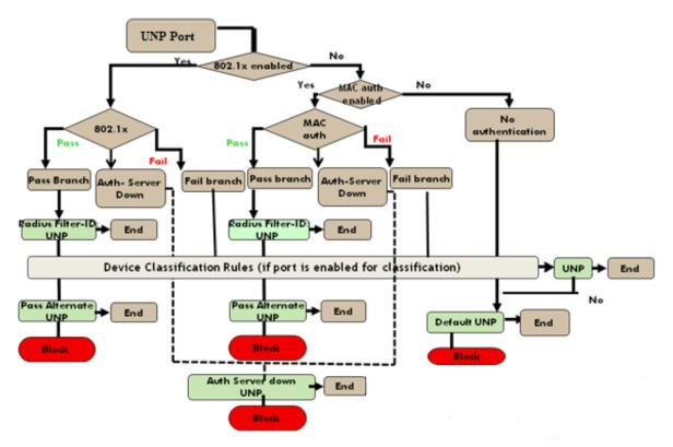
Figure 35-2 : UNP - Device authentication and classification process
