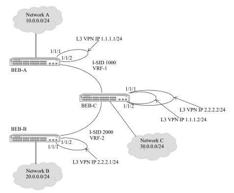
Figure 7-23 : IPv4 Inter-ISID Routing Example (Two VRFs)
