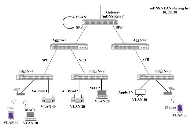
Figure 35-21 : mDNS Gateway - mDNS Devices Connected to an SPB Domain
