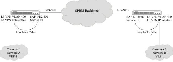
Figure 7-10 : L3 VPN Interface: External Loopback
