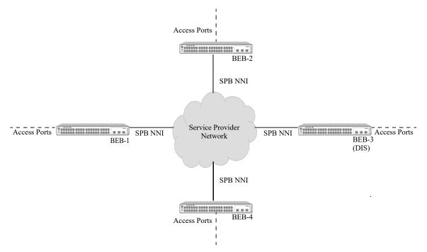
Figure 7-11 : SPB Backbone over a Service Provider Network
