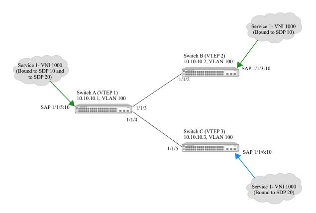
Figure 17-5 : Sample VXLAN Configuration with no Routing Framework
