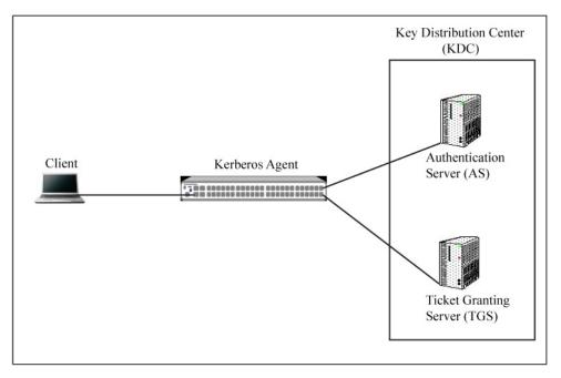
Figure 38-3 : Kerberos Snooping Authentication
