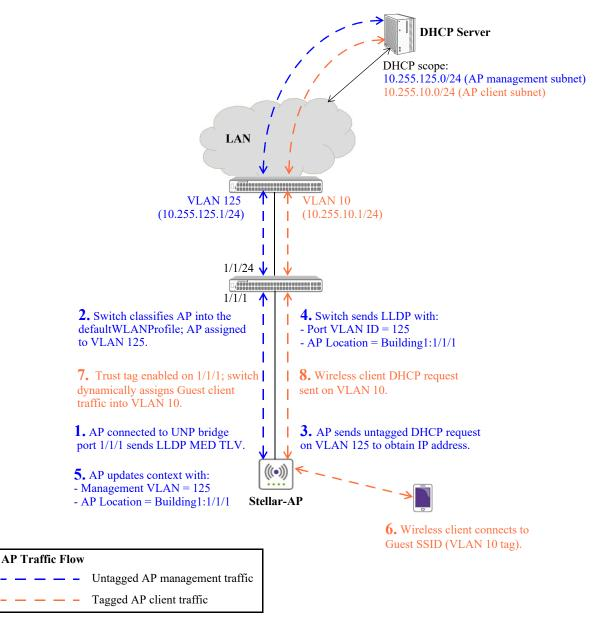
Figure 35-7 : OmniSwitch AP Discovery and Integration Example - VLAN Domain
