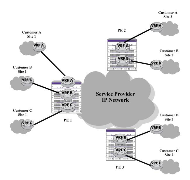
Figure 22-1 :Example Multiple VRF Configuration
