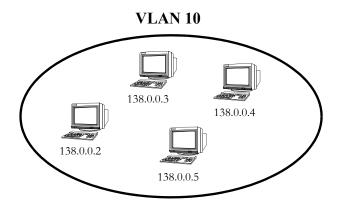
Figure 4-3 : VLAN Bridging Domain: Logical View
