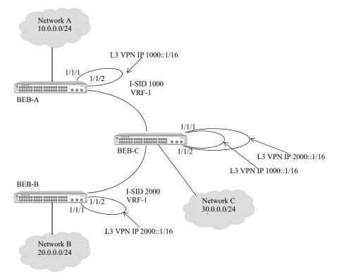
Figure 7-22 : IPv6 Inter-ISID Routing Example (One VRF)
