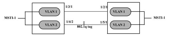
Figure 6-10 : Automatic VLAN Containment - AVC enabled
