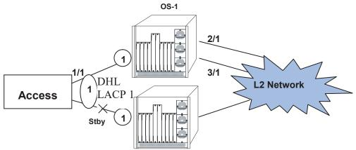
**Figure 1-1 : Link Fault Propagation - Application Example**
