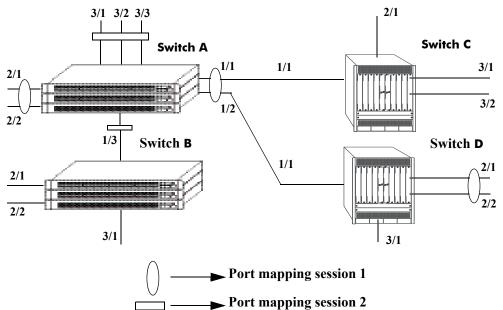
Figure 39-1 : Example Port Mapping Topology
