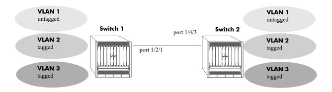
Figure 4-1 : Tagged and Untagged Traffic Network
