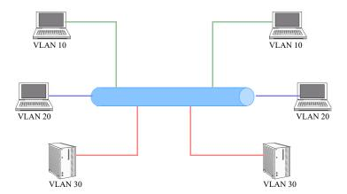
Figure 7-16 : Devices Remotely Connected on a Pseudo-Wire
