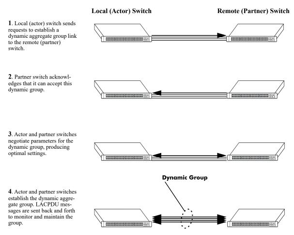
Figure 10-1 : Example of a Dynamic Aggregate Group Network
