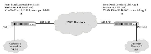
Figure 7-9 : L3 VPN Interface: Inline Routing (Front-Panel Ports)
