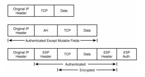
Figure 24-1 : IP Packet in IPsec Transport Mode
