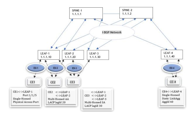
Figure 18-8 : EVPN on VXLAN Service - Configuration Example
