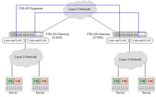
Figure 17-1 : OmniSwitch VXLAN Gateway Example
