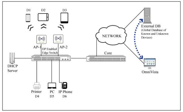
Figure 35-26 : IoT Example - OV interaction with OmniSwitch
