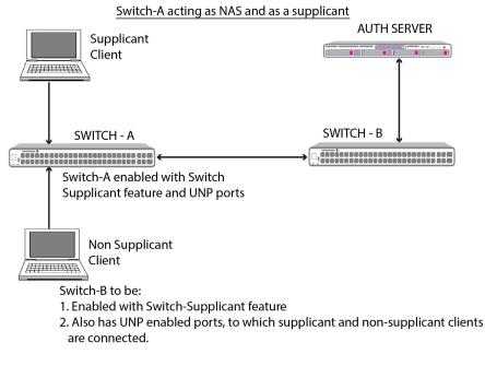
Figure 35-10 : Switch-A acting as NAS and as a supplicant
