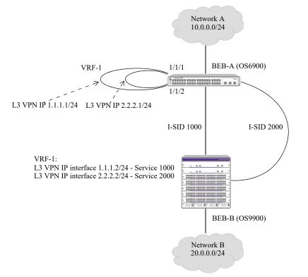
Figure 7-20 : IPv4 L3 VPN External Loopback and Service-based Interfaces
