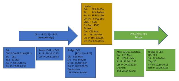
Figure 18-2 : The Inter EVI Packet Forwarding in Asymmetric IRB Based EVPN Network
