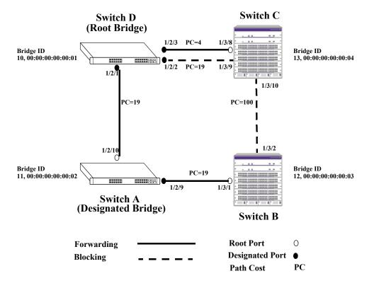
The following diagram shows the logical connectivity of the same physical topology as determined by the Spanning Tree Algorithm:
