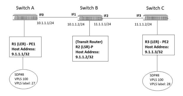
Figure 16-3 : VPLS with Signaling BGP Configuration Example
