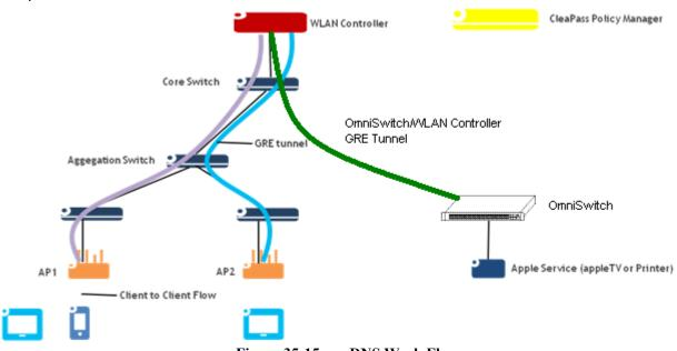
Figure 35-15 : mDNS Work Flow
