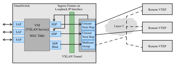
Figure 17-2 : OmniSwitch VXLAN Service Components
