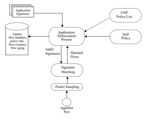
Figure 36-2 : Application Enforcement Process
