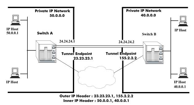
**Figure 21-6 : Tunneling Operation**
