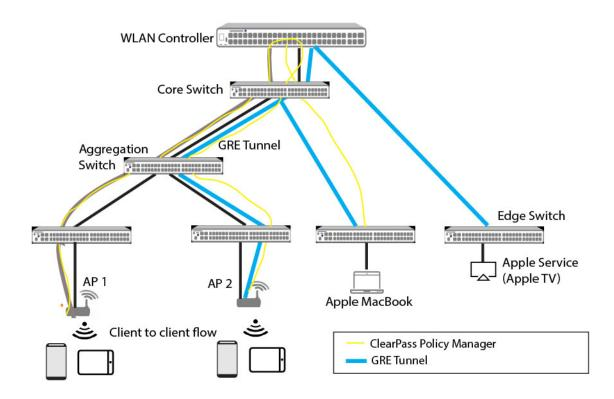
Figure 35-18 : Zero Configuration Networking - Aruba Mode
