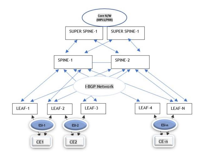
Figure 18-7 : 3-Tier EVPN-VXLAN Network Based on a Spine and Leaf Deployment with the Super-Spine Node
