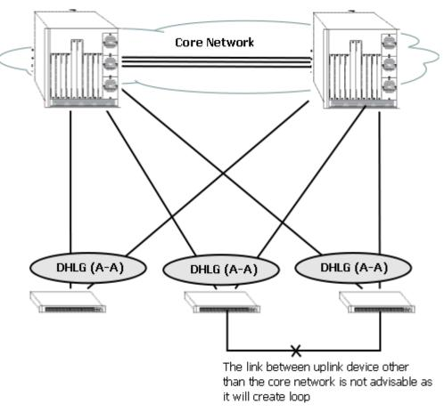
Figure 11-4 : Unsupported DHL Active-Active Topology (Network Loops)
