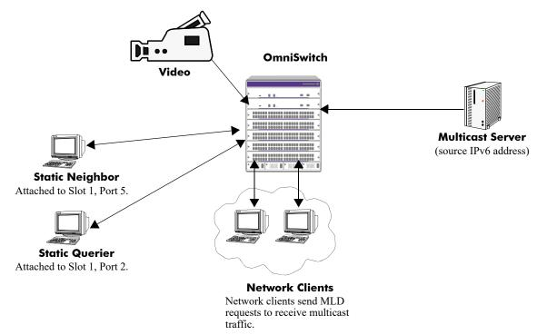
Figure 31-4 : Example IPMS v6 Network
