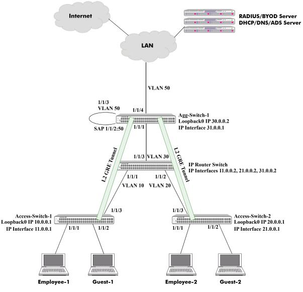
Figure 35-9 : OmniSwitch L2 GRE Tunneling Configuration Example
