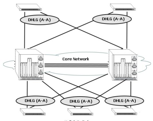
Uplink Switches Figure 11-3 : Recommended DHL Active-Active Topology
