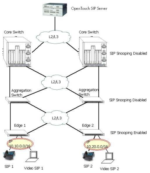
Figure 20-2 : SIP Snooping Use Case
