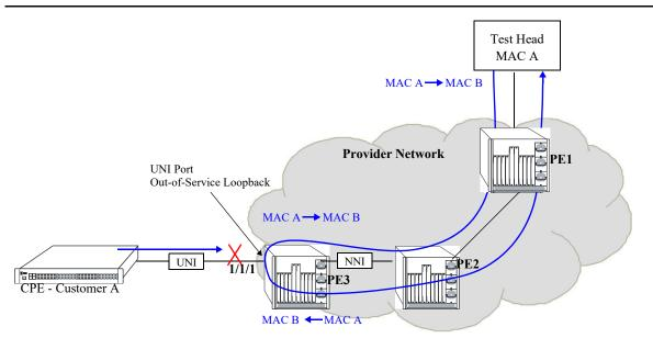
Figure 42-3 : Outward (Egress) Loopback Test Example
