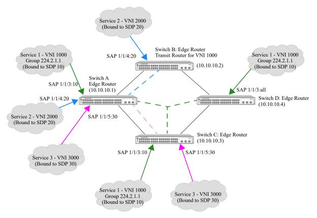
Figure 17-3 : Sample VXLAN Configuration with Static Routes
