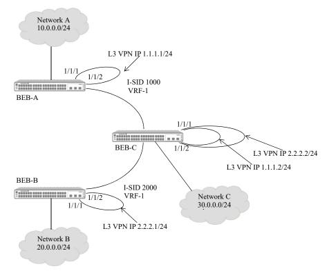
Figure 7-21 : IPv4 Inter-ISID Routing Example (One VRF)
