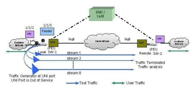
Figure 46-4 : Configuring a CPE Test Group Profile
