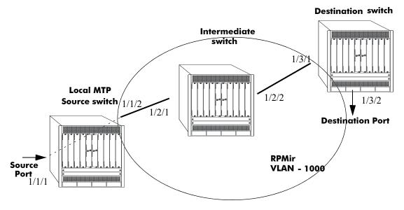
**Figure 41-3 : Remote Port Mirroring Example**
