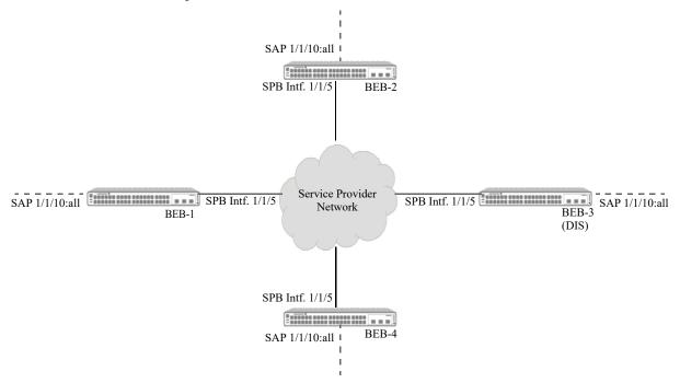
Figure 7-27 : SPB Backbone over a Shared Network
