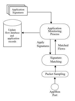
Figure 36-1 : Application Monitoring Process
