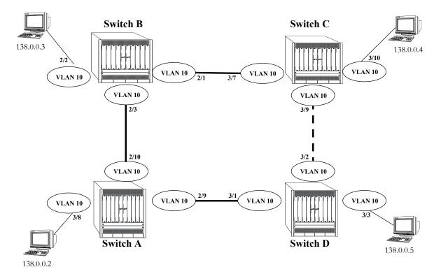
Figure 4-2 : VLAN Bridging Domain: Physical Configuration
