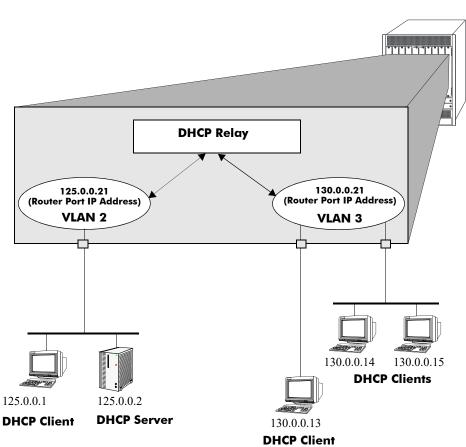
Figure 27-2 : DHCP Clients in Two VLANs
