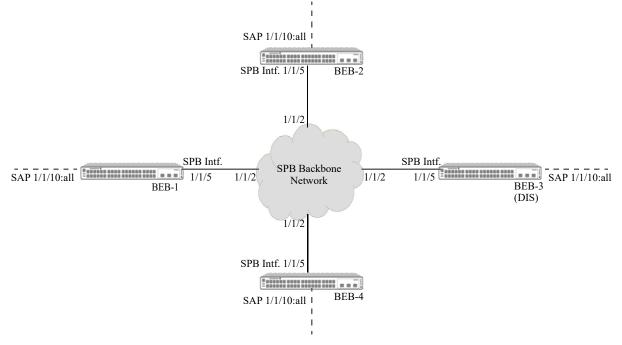
Figure 7-28 : SPB Backbone over Another SPB Network
