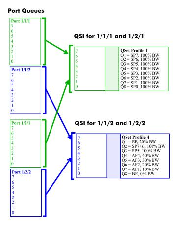
Figure 33-2 : Queue Set (QSet) Framework (Unicast Traffic)
