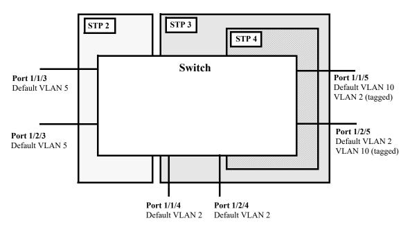
Figure 6-8 : Per VLAN (single and 802.1Q) Spanning Tree Example
