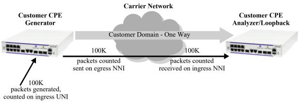
Figure 46-1 : CPE Test Head Example - Unidirectional, Ingress Test
