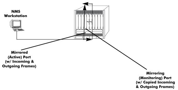
Figure 41-1 : Relationship Between Mirrored and Mirroring Ports
