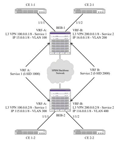
Figure 7-18 : IPv4 L3 VPN Service-based Interfaces (Inline Routing)
