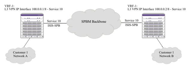
Figure 7-8 : L3 VPN Interface: Inline Routing (Service-Based IP Interface)
