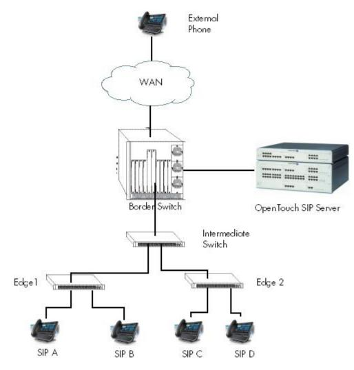
Figure 20-1 : Using SIP Snooping
