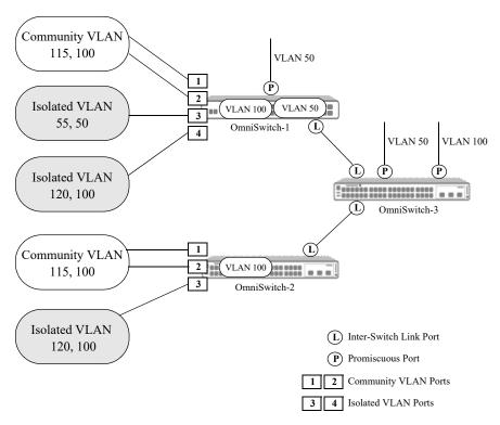
Figure 4-5 : PVLAN Spanning across Multiple Systems
