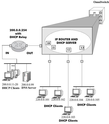
Figure 28-1 : Internal DHCP Server Application Example
