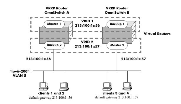
Figure 29-4 : IPv6 VRRP Redundancy and Load Balancing
