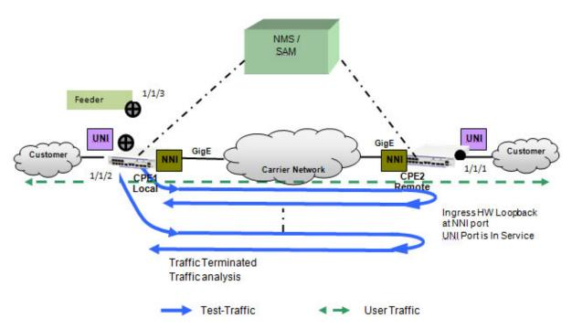
Figure 46-7 : Sample Bidirectional Multi-stream Test Configuration
