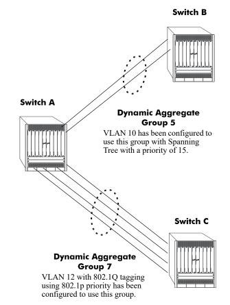
Figure 10-2 : Sample Network Using Dynamic Link Aggregation
