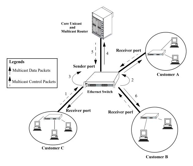
Figure 32-1 : Packet Flow in the VLAN Stacking Mode
