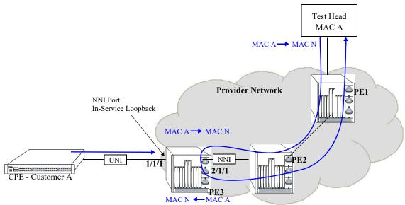
Figure 42-4 : Inward (Ingress) Loopback Test
