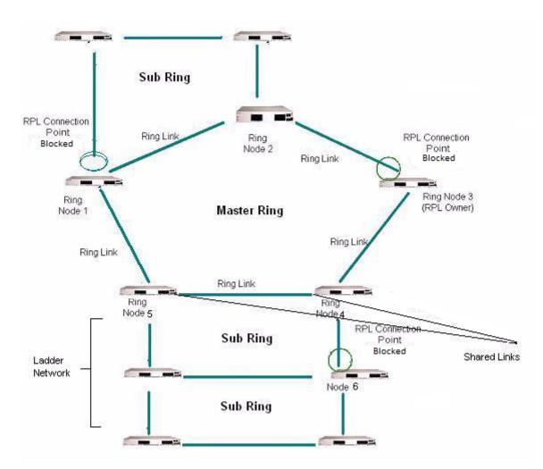
Figure 12-3 :ERPv2 on Multi Ring and Ladder Network with RPLs and Shared Links
