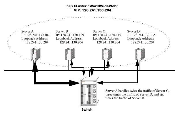
Figure 30-2 : Weighted Round Robin Algorithm
