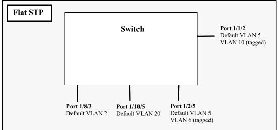
Figure 6-7 : Flat Spanning Tree Example
