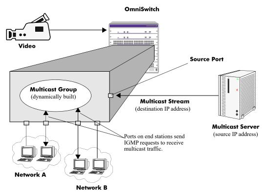
Figure 31-1 :Example of an IPMS Network
