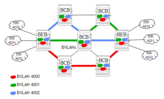
Figure 7-1 : SPBM Network Components
