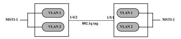
Figure 6-9 : Automatic VLAN Containment - AVC not enabled
